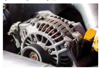
is not working properly. For example, the radio, lights, and automatic windows are powered directly from the alternator in most vehicles. If the alternator is faulty, the battery will discharge very quickly, almost in the course of driving.
